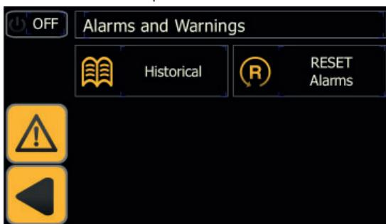
When the nominal working conditions have been restored, some warning and alarm are automatically reset, for other alarms/warning it is necessary to perform a manual reset.
